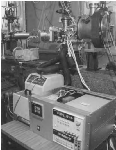
Figure 1: Schematic drawing and photo of MICROCALIX setup (photo taken at LURE D24 station). RX coming from left are passing through the calorimeter cell and its sample capillary-contained. Cryostat assures T control, while calorimeter electronics (facing in photo) and PC computer simultaneously collect DSC and X-ray data thank to PSDs.
