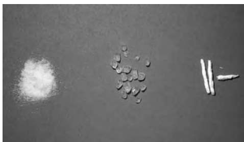
Figure 4: Examples of extrudate shapes: extrudate powder (left), granules (middle) and strands (right).
